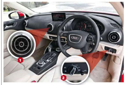
Thin pop-up screen can be switched off manually and provides a whole range of info, ranging from multimedia to sat-nav
