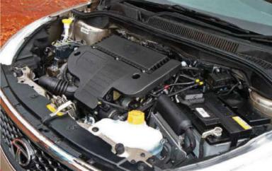
A Familiar Quadrajet turbo-diesel motor takes pride of place, armed with 200 Nm of torque
