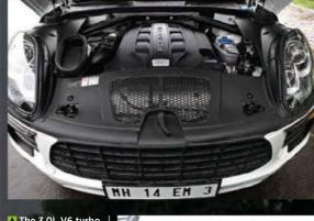
The 3.0L V6 turbo diesel pulls cleanly without the slightest hint of lag despite the forced induction at work
