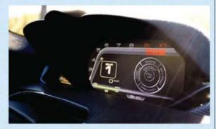
what initially appears to be Ferrari's usual dial pack consisting of a traditional analogue and secondary TFT displays. But this time the whole lot is TFT, and can be configured to show engine speed on a conventional circular gauge, or on a horizontal scale that looks like an Astra GTE-owner's wet dream.
